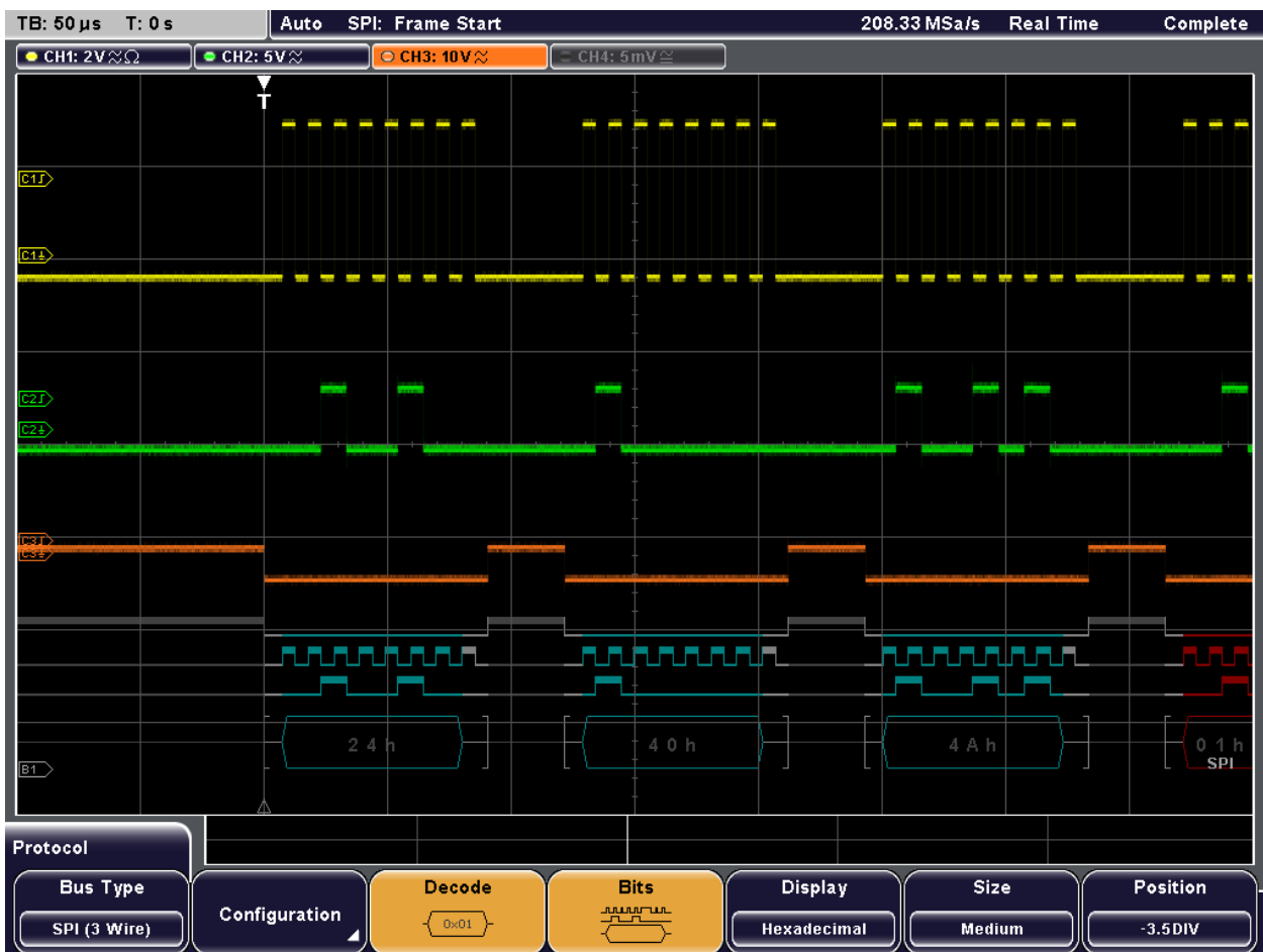
Fig. 11-2: Decoded SPI signal
